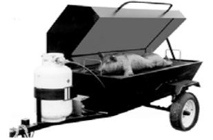
2. To light the pig roaster, turn control knob to PILOT POSITION. Depress control knob and repeatedly press red igniter button until the pilot is lit. Continue depressing the control knob. Sufficient time must be allowed for the thermocouple to heat and hold the safety magnet in a locked position. Turn control valve to ON. After burner ignites, allow the roaster 10-15 minutes to heat up to a desired temperature.
